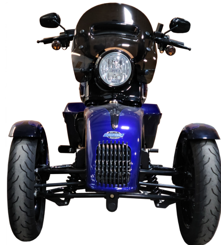
TiltLock turned ON (motorcycle is held upright by TiltLock, kickstand not in use)
